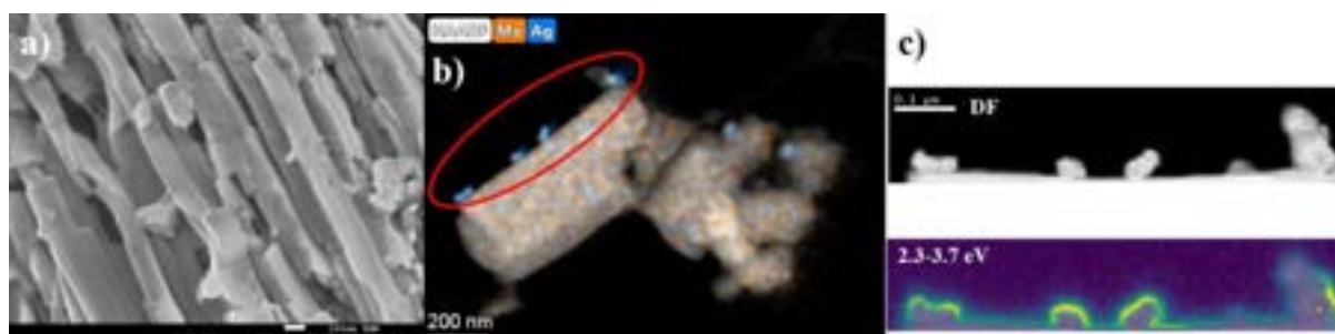
Figure 1: a) SEM Image of the (TBA) 2 Ag 2 [Mo 8 O 26 ] nanowires, b) Superposition of TEM micrograph and EDS elemental maps. The red circle highlights the area used to acquire the EELS data c) Dark field (DF) image (DF) and EELS plasmonic maps acquired in the energy range 2.3-3.7 eV.
